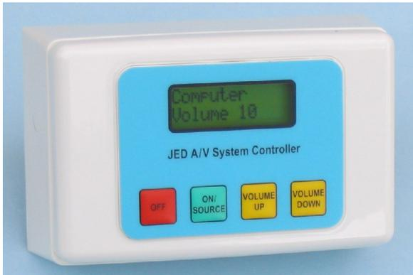
The *JED AV System Controller* connects to your installed projector using a data cable which allows RS232 communication between the controller and projector. When a user of the system presses the On/Source button, a code is sent to the projector which is effectively the same as pressing the power button on the projector case.
